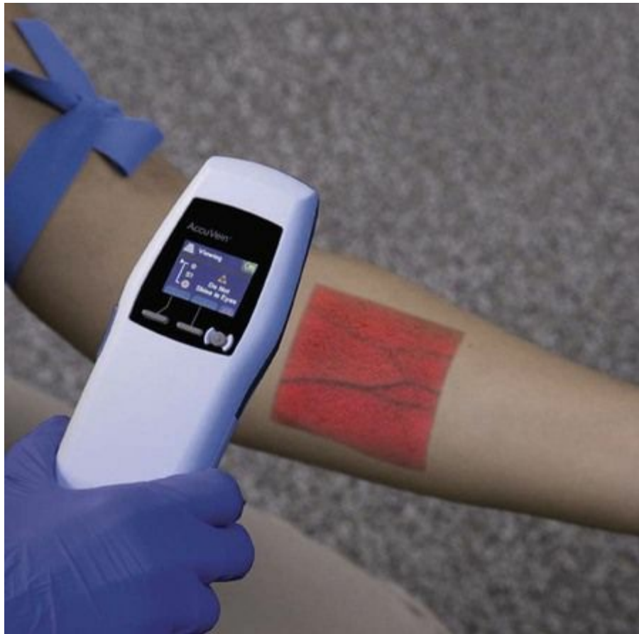
FIG. 13-3 The AccuVein AV300 is a vein illumination device that helps health care professionals locate veins for blood draw, IV infusion, and blood donation by projecting a pattern of light on the patient's skin to reveal the position of underlying veins on the skin's surface. The device uses red and infrared light, which the hemoglobin in blood absorbs to detect the position of the vein.
