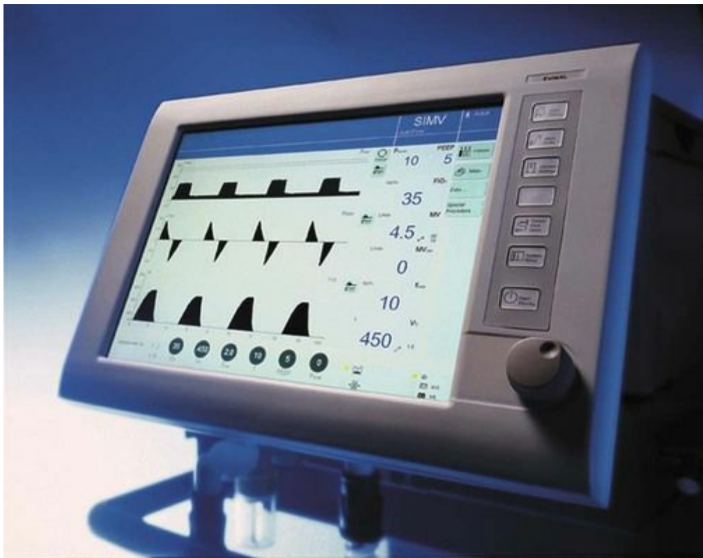
FIG. 32-3 Display signals, alarms, and control panel of a typical volume-cycled ventilator.
