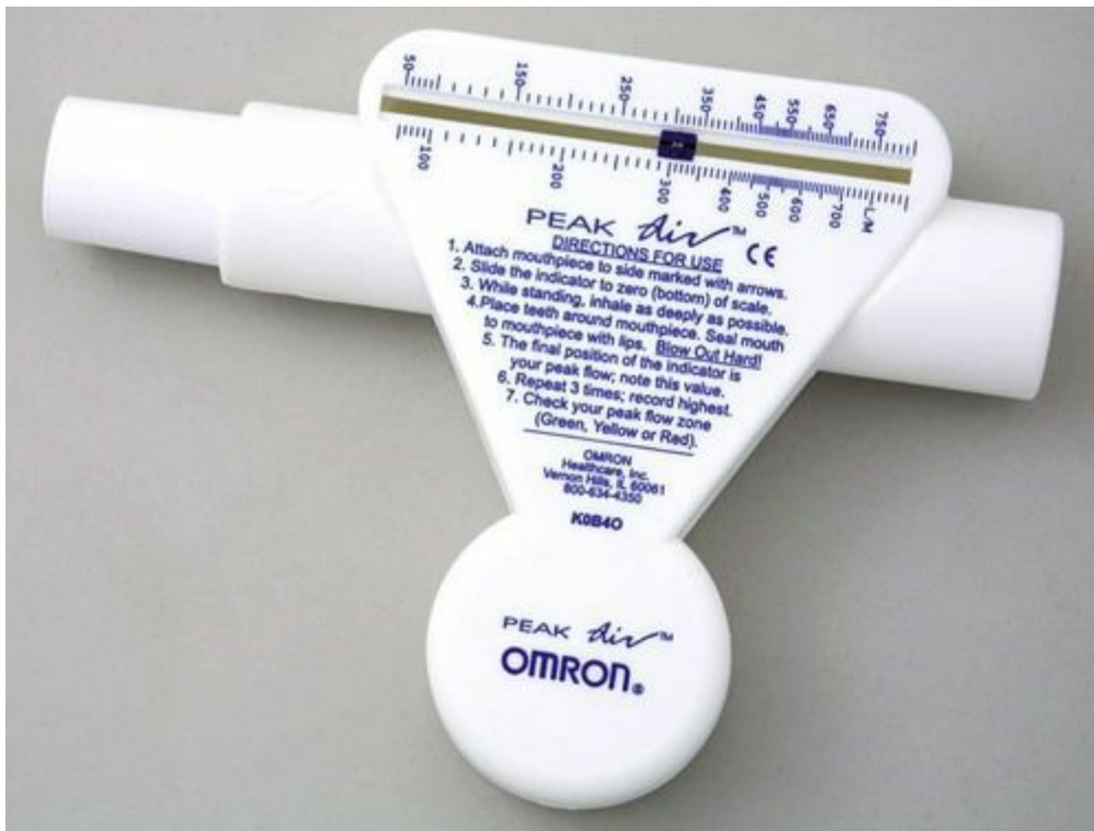
FIG. 30-4 A typical peak flowmeter. This model will show faster exhalation rates in green , reduced exhalation rates in yellow , and seriously reduced exhalation rates in red .
